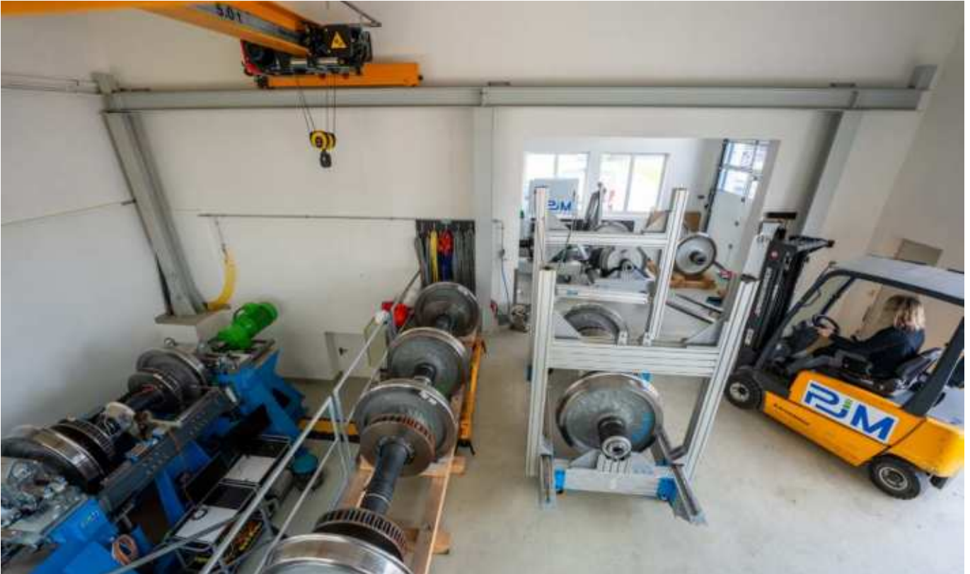
The infrastructure in the field of instrumented wheelsets includes a stationary test rig, a dynamic test rig and the corresponding technical equipment such as an indoor crane Credit: Manuel Hanschitz for PJM, free of charge
