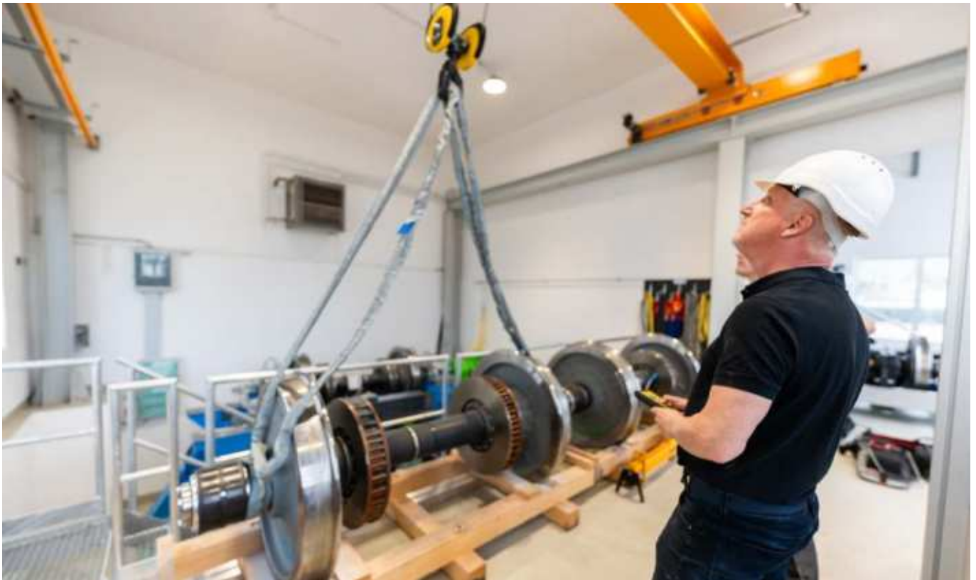
PJM handles all processes and project steps relating to instrumented wheelsets in-house and from a single source: calculation, design, production, calibration and balancing Credit: Manuel Hanschitz for PJM, free of charge
